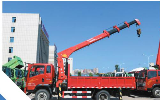
随车吊 Truck Mounted Crane
